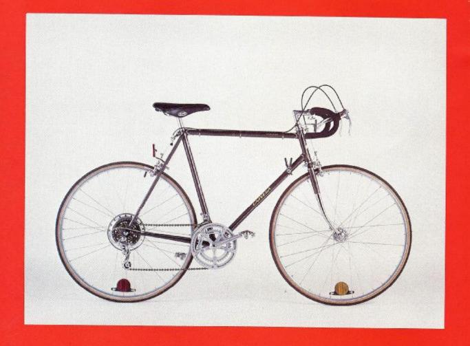
HAND BUILT WITHOUT ANY COMPROMISE, FOR HIGH PERFORMANCE TOURING, HI Tension double butted tubings throughout, special rear stays, Cinelli type fork crown, professional type forged light alloy crankset, alloy wheels, with SUNTOUR CYCLONE derailleur. See specifications for more detail and compare the difference.
