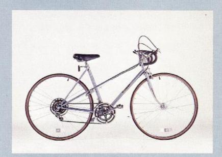
A TRUE SUPER VALUE, WITH DURABILITY AND GREAT LOOKS. Fully lugged frame, alloy cotterless crank, 27" wheels with alloy hubs and SUNTOUR SEVEN 10 Speed. See specifications for more details.
